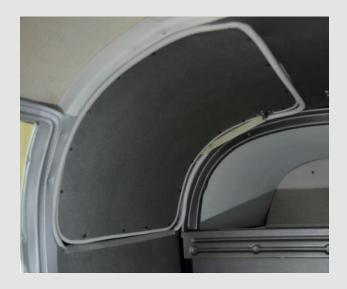
To assure cracks do not return, make certain plastics are not forced into place. Rather trim the curved edge of a door panel or simply eliminate unneeded screws. Baggage door liner problems can be resolved by fitting a new one.
