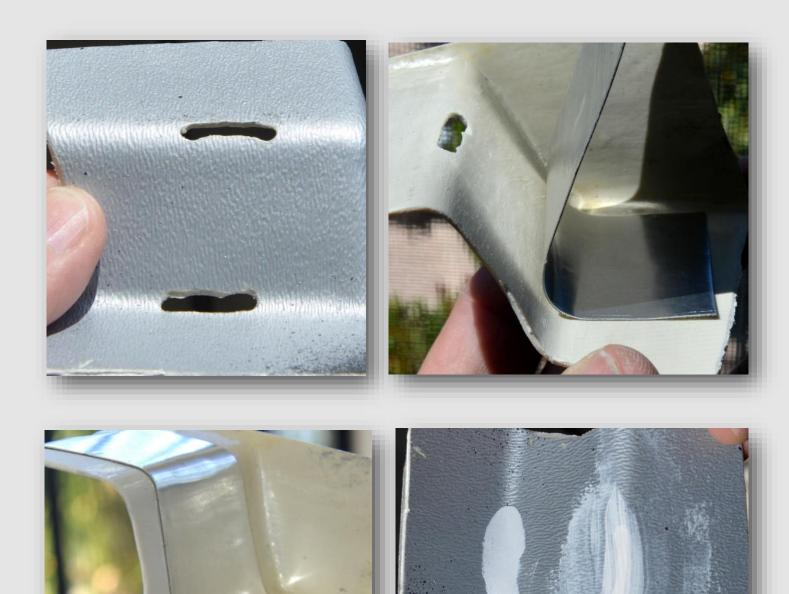
Soft aluminum acrylic tape patch forms easily to precisely cover blemishes. PlasticWeld totally fills voids and when sanded leaves a near invisible repair.
