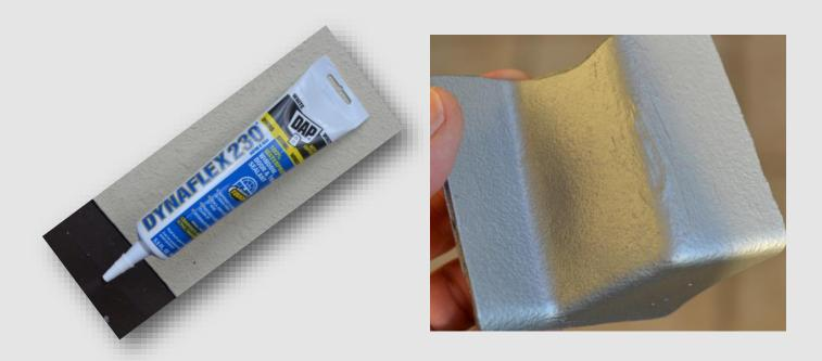
Disappointing reoccurring cracks due to flexing during install, can be eliminated by use of a paintable caulk, such as DAP Dynaflex 230. Applied directly from the tube and profiled with stiff shortened bristles from a 1 inch paint brush, provides a finished look. Complete the job with primer, aerosol truck bed, colors and protective top coats.
