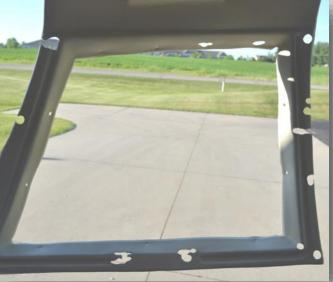
After scrub cleaning, profile every blemish with a Dremel pointed grinding bit keeping edge openings to a minimum. Acrylic patch repair creates a void to be filled. Prepare underside by scuffing with coarse sandpaper and cleaning with plastic prep.
