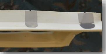
Blemishes totally removed with Dremel grinding bit keep openings to a minimum. Backside sanded and prepped, foil patches quickly cover blemishes.
