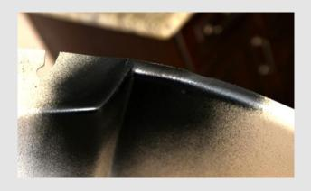
Truck bed aerosol texture applied to repairs further enhances the area. Multiple coats will assist in filling any remaining blemishes. Coat with primer to assure consistent luster
