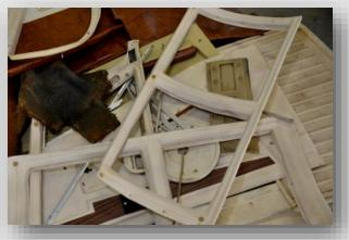
With eyeball vent headliner in place, apply plastic prep aerosol and scrub with Scotch Brite pad. Wipe with soft cloth and mask as needed. Before applying aerosol finishes, repair blemishes as described in the following pages.
