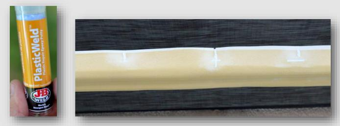
PlasticWeld fills voids and when sanded smooth is ready to receive adhesion promoter, texture, color and protective finishes. Use minimal amount and thoroughly mix two-part epoxy massaging with moisture to keep from sticking to your fingers until achieving a consistent color. Once applied and cured, sand until all PlasticWeld is removed from the original surface.
