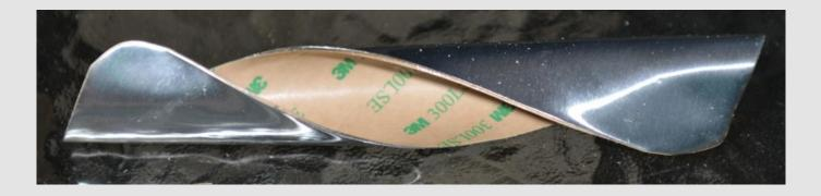
Soft aluminum .016 foil and acrylic transfer tape very effectively cover typical blemishes from pulled through screws, aging and heat damaged plastics. Cut with a scissors, this easily formed material precisely profiles to the mating surface. Round corners for better adhesion.
